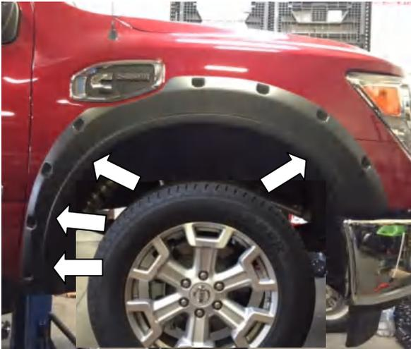
**STEP 7:** Place Fender Flare on vehicle, ensure the slots in the Fender Flare align with the holes in the wheel arch from the previously removed factory screws. Using #2 Phillips head screwdriver, re-install the previously removed (4) screws through slots in Fender Flare. Once positioned correctly ensure all fixing points are tight and secure.
