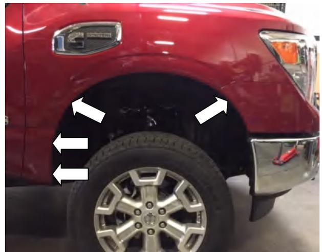
**STEP 6:** Place Fender Flare on the vehicle into the position of best fit. Note where (4) slots in Fender Flare correspond with existing screws / fixing points in the wheel arch. Remove Fender Flare. Remove any existing vehicle screws in locations as shown with #2 Phillips head screwdriver. Maintain screws for re-installation.
