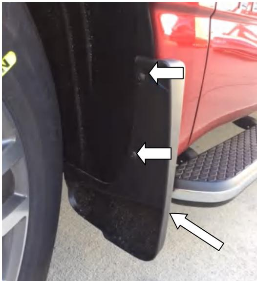
**STEP 5:** For vehicles equipped with factory mud guards. Remove (3) retaining screws to remove mud guard. Store mud guard in a safe place, it will not be re-used for Fender Flare installation. Reinstall screw in underside rocker panel area and retain (2) remaining screws from inner wheel arch for Fender Flare Installation.
