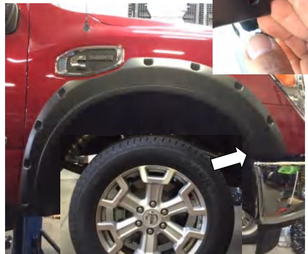
**STEP 8:** Install the provided U shape metal clip at the (1) remaining slot location in the Fender Flare. Ensure that positive pressure is applied on the Fender Flare to the vehicle fender when installing clips. Slide the clip over the Fender Flare and the inner lip of the front bumper fascia ensuring that the barb in the clip locates in the slot of the Fender Flare. Ensure that the rubber seal is flush neatly against the vehicle body.
