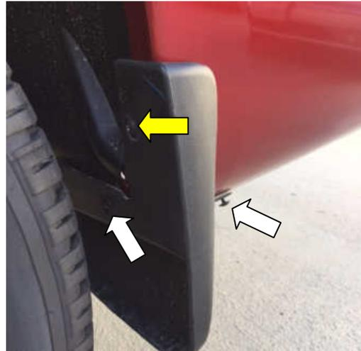
**STEP 9:** Clean the body area where the Fender Flares will make contact. Ensure fenders are dry prior to install. For models equipped with factory fender flares, removal of factory flares is required, please consult the vehicle service manual for factory fender flare removal.
