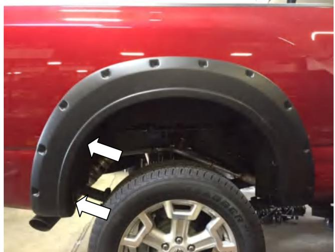
**STEP 11:** Place Fender Flare on the vehicle into the position of best fit. Note where (2) slots in rear of Fender Flare correspond with existing screws / fixing points in the wheel arch. Remove Fender Flare. Remove any existing vehicle screws in locations as shown with #2 Phillips head screwdriver. Maintain screws for re-installation.
