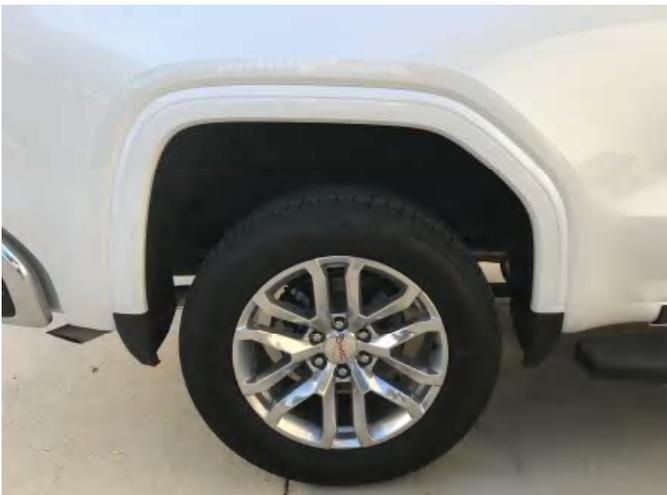
**STEP 10:** Clean the body areas where the Fender Flares will make contact. Ensure fenders are dry prior to install.
