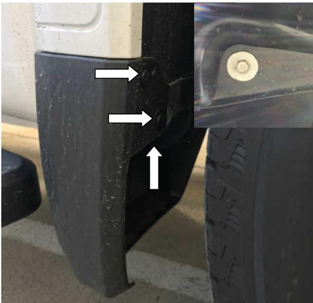
**STEP 5:** Using #15 Torx head screwdriver remove the upper and lower screws from the front factory mudguards and using M10 socket remove the underside screw indicated above, maintain #15 Torx head screws for re-install. Fender flares require the mud guards to be removed. Retain factory mudguards for later use if required.
