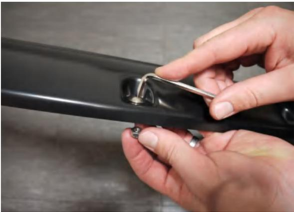
**STEP 1:** Attach the bolts and nuts to each Fender Flare using a 3/16" Allen key/Trox and a 1/2" wrench/socket. (wrench /socket and Allen key not supplied). Ensure inside of Fender Flares where the rubber seal is attached is clean, using the alcohol wipes provided. Wipe away any residue with a dry clean cloth.
