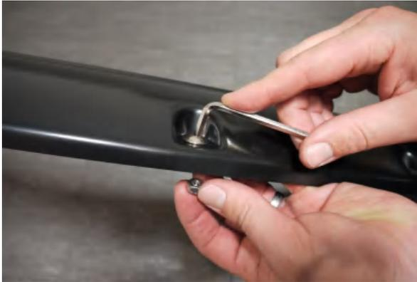
**STEP 8:** Attach the bolts and nuts to each Fender Flare using 3/16" Allen key/Trox and a 1/2" wrench/socket. (wrench /socket and Allen key not supplied). Ensure inside of Fender Flares where the rubber seal is attached is clean, using the alcohol wipes provided. Wipe away any residue with a dry clean cloth.
