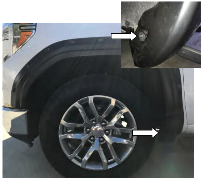
**STEP 6:** Place Fender Flare on the vehicle into the position of best fit. Using #15 Torx head screwdriver re-install previously removed factory mudguard screw at the lower screw location through the slots in the Fender Flare at the noted location.
