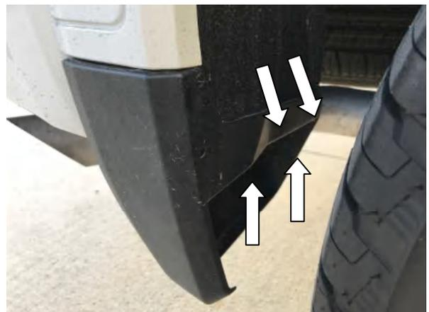
**STEP 11:** Using #15 Torx head screwdriver remove the two upper and two underside screws from the rear factory mud guards in the rear wheel arch. Fender flares require the rear mud guards to be removed, maintain screws for re-install if required.
