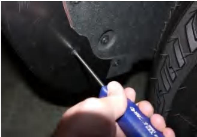
**STEP 9:** Re-install factory screw in the mudguard using #15 Torx head screwdriver through the slot in the Fender Flare.
