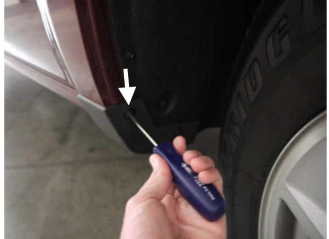
**STEP 6:** Using #15 Torx head screwdriver remove upper screw from the front factory mudguard. Maintain screws for re-install.
