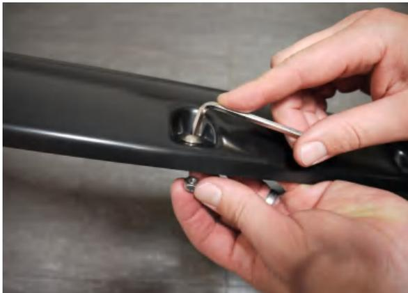
**STEP 1:** Attach the 10 bolts and nuts to each Fender Flare using a 3/16" Allen key and a 1/2" wrench/socket. (wrench /socket and Allen key not supplied). Ensure inside of Fender Flares where the rubber seal is attached is clean, using the alcohol wipes provided. Wipe away any residue with a dry clean cloth.
