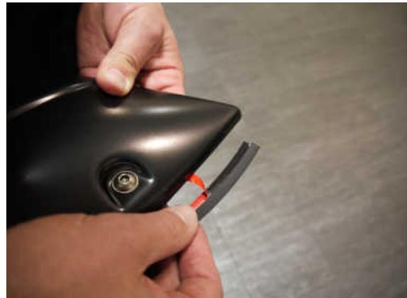
**STEP 2:** Attach the included rubber seal to the Fender Flares. Peel back 2" of the adhesive backing and position on the Fender Flare. Attach the seal to the Fender Flare, peeling back a few inches at a time. Ensure pressure is used to secure rubber seal to Fender Flare edge. Attach rubber seal along all areas the Fender Flare will make contact with the vehicle body.
