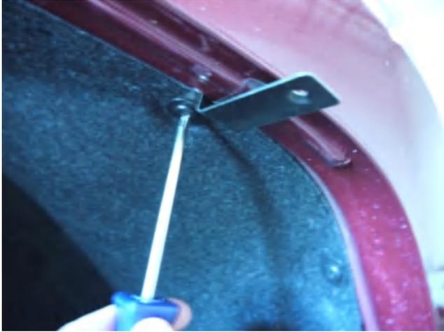
**STEP 7:** Apply clear tape to the inside edge of the fender wheel arch in front of positions **A** and **B** (step 5) over mastic sealant. Install the large brackets in positions **A** and **B** (step 5) aligning the slot in the bracket with the vacant holes from the factory screws in the vehicle wheel arch. Ensure clips are positioned over the clear tape. Re-install the factory screws in location **A** and **B** using a #15 Torx head screwdriver.
