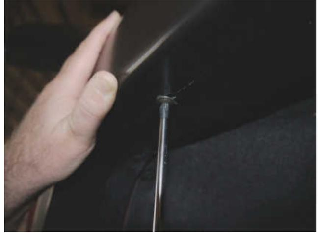
**STEP 8:** Place Fender Flare on the vehicle into the position of best fit so the slots in position **A** and **B** are over the holes in the front end of large clips. Ensure bottom rear slot in Fender Flare is located over the vacate hole in the factory mudguard. Apply upward tension on Fender Flare to the vehicle fender when installing the screws and washers provided into the clips in position **A** and **B** using a Philips head screwdriver.
