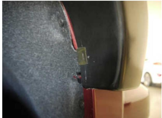
**STEP 10:** To secure the front slot in the Fender Flare to the body, take the black metal clip and slide it over the Fender Flare and the inner wheel arch lip. Position the clip so that the barb in the clip locates in the slot of the Fender Flare. Ensure all fixing points are tight and secure and that the rubber seal is flush neatly against the vehicle body.
